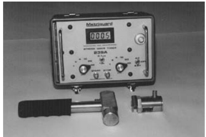
Figure 7—Metriguard Model 239A Stress Wave Timer.
